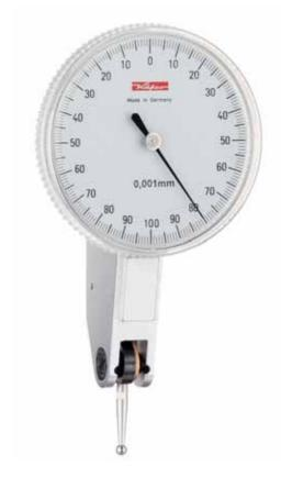
Another Dial Test Indicator with a reading of 0.001 mm is our model K 58. This model provides excellent readability due to its bezel diameter of 58 mm.
